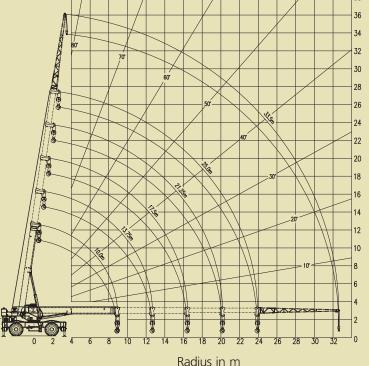
Lifting Capacities for supported operation only on firm level ground. Weight of 40T hook block=450 kgs. Lifting capacity= actual load+ hook block +Lifting equipment. With boom extension assembled, ratings shown will be reduced. These lifting capacities do not exceed 85% of the tipping load.
