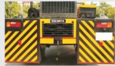
Rear view camera and integrated protected tail lights. High ground clearance.
