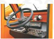
Steering Wheel Articulated power steering controlled through steering wheel for safe usage and precision control
