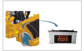
Heavy duty, maintenance free battery at convenient location - 180 Ahr
